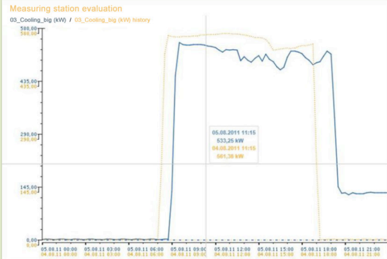
Illustration 9: Comparison of a daily load curve of a cooling system (graphical) [Source: Vattenfall]
